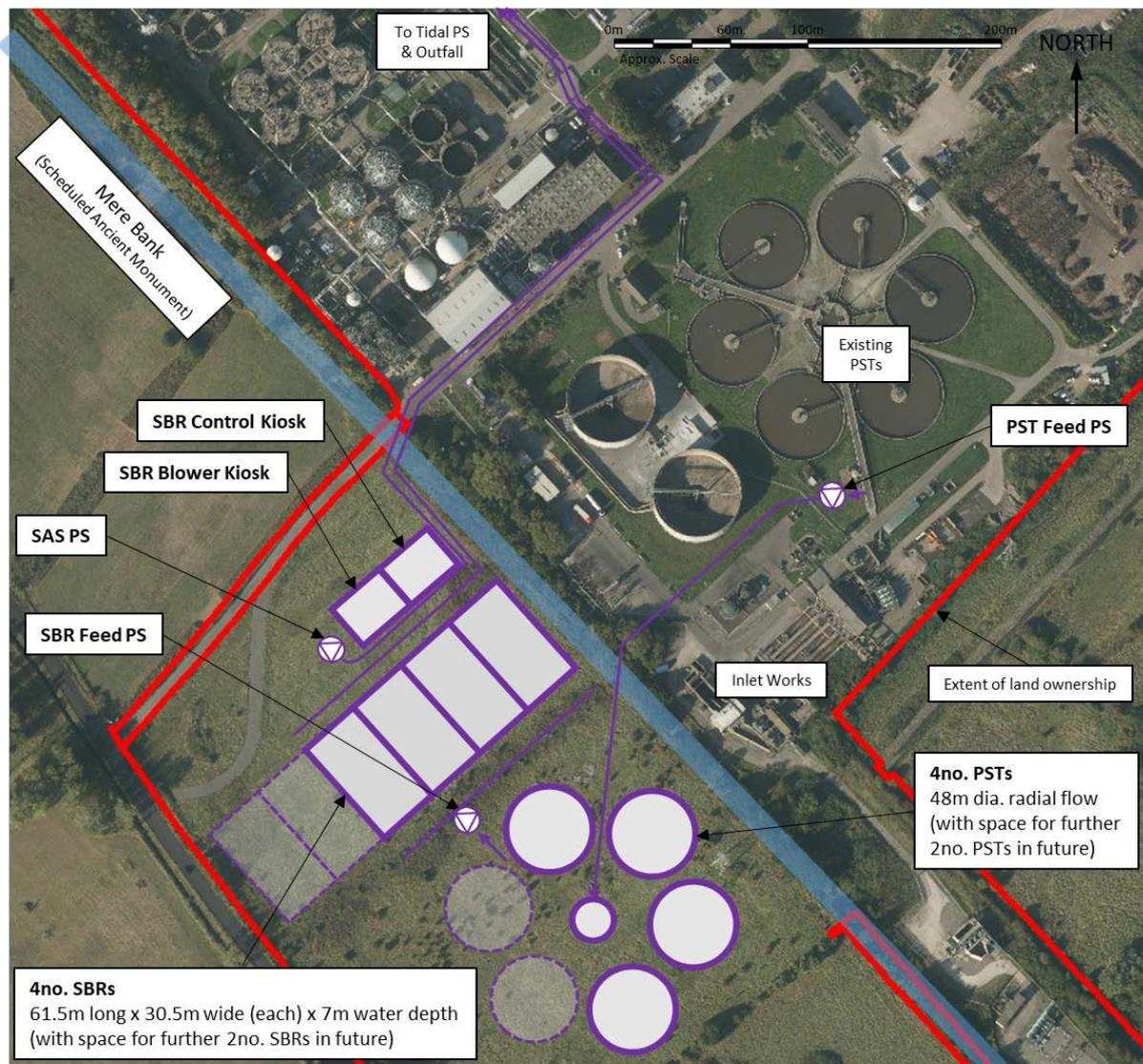
Due to the requirement under the WINEP, a significant increase in hydraulic capacity is required at the works. The hydraulic capacity enhancement will additionally provide treatment capacity enhancement up until 2025. Following this it is expected the permitted
